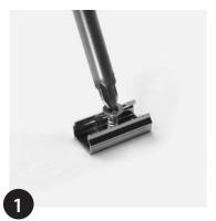
Fix clips with suitable screws (min. 2 per metre/40").
